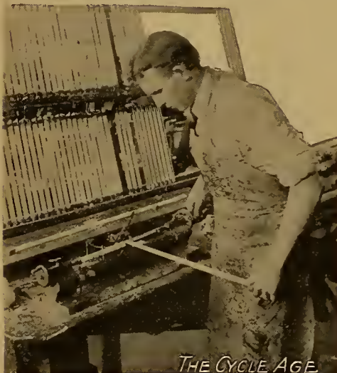
Running Paper Strip Onto Gang of Rings.
